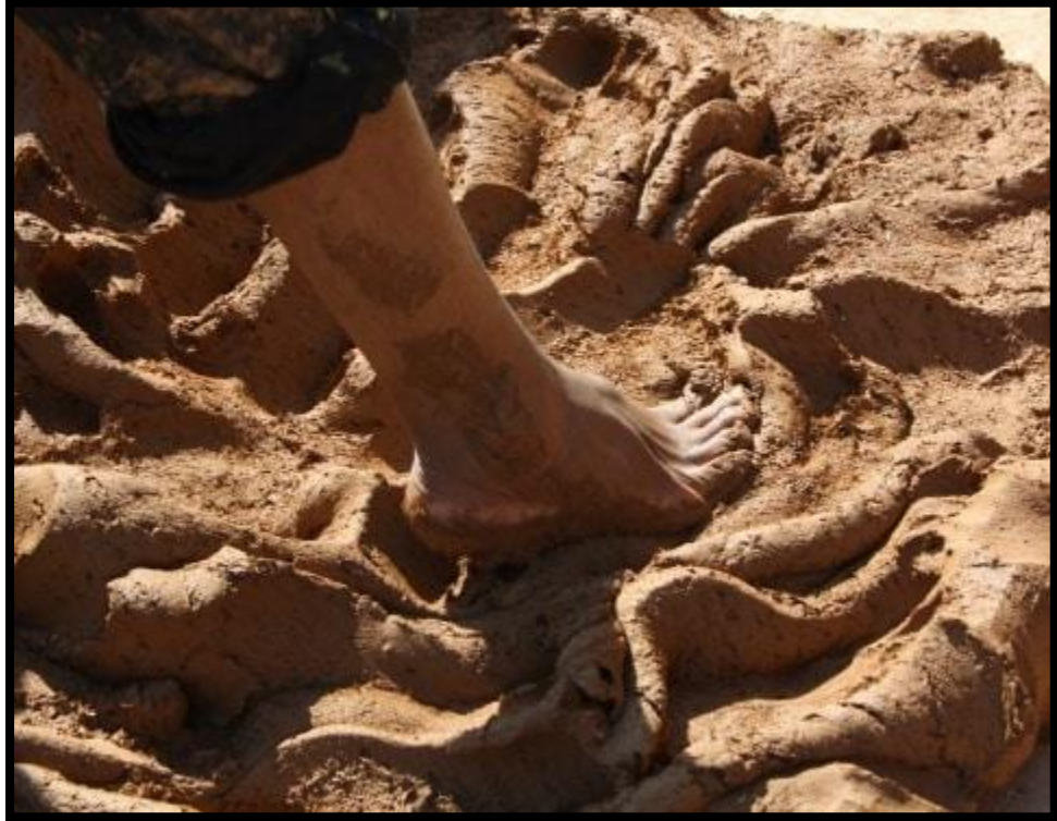
Molding of clay for brick manufacturing
