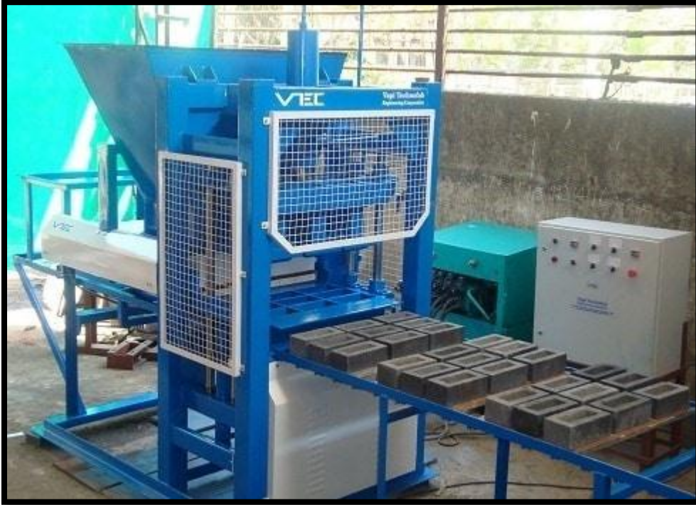
Machine molding of bricks
